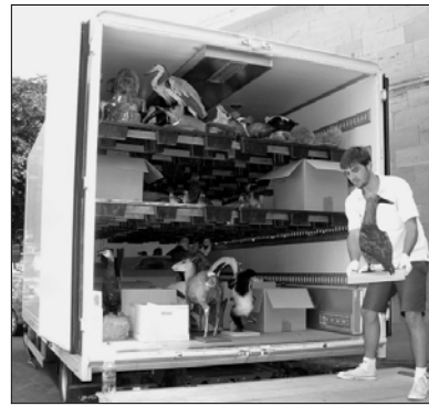
Figure 4. Mobile Thermo Lignum heat chamber.
